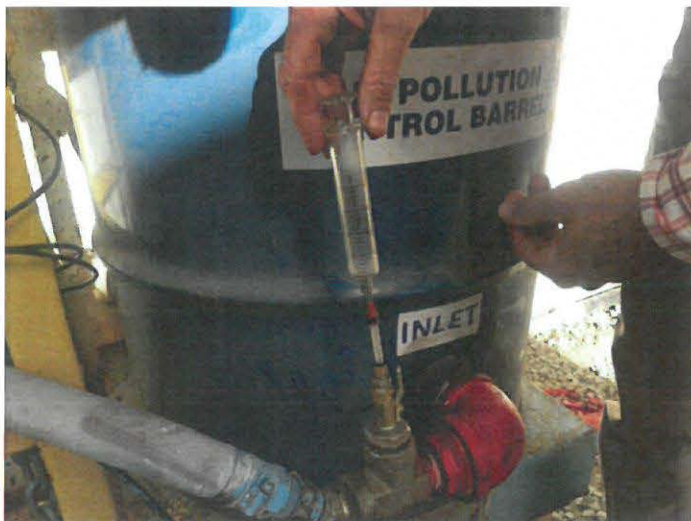
Figure 4 . Sampling port with gas sampling syringe connected through septum.
