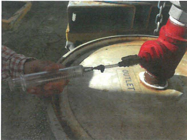
Figure 3. Sampling port with gas sampling syringe connected through septum.
