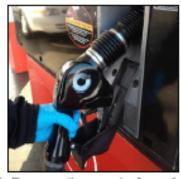
Remove the nozzle from the dispenser cradle without touching the lever. If the hold-open latch is engaged, the nozzle fails. The nozzle shall not be used and must be immediately taken out of service.
